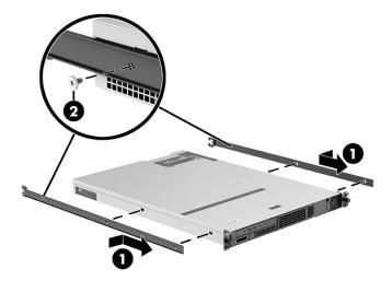
3. Slide the computer into the rack, being sure to place the glides into the rails.
