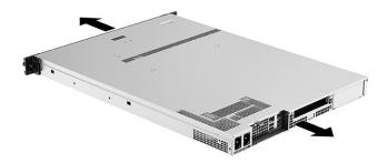
⚠ WARNING! Be sure that the ambient air temperature is within specified limits. To locate specifications for your computer, see Product specifications on page 7.
